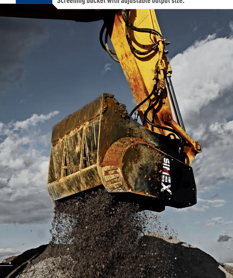
■ Designed for **separating different-sized materials** on the work site.
